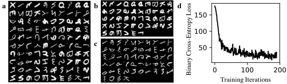
Figure 11. Training of a binary classifier to discriminate between bold and thin letters. a. Training set of the EMNIST dataset including bold and thin letters. Output of the trained network of letters labelled as b. bold and c. thin. d. Loss curve corresponding to the training of the binary classifier.
