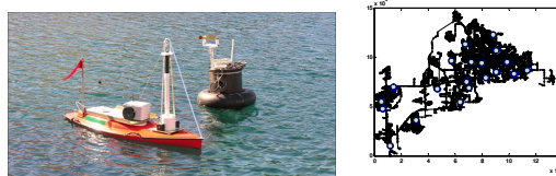
Figure 1: (a) Monitoring Lake Fulmor [courtesy of NAMOS ( http://robotics.usc.edu/~namos ) & CENS ( http://cens.ucla.edu )]; (b) Water network sensor placement in BWSN challenge.
