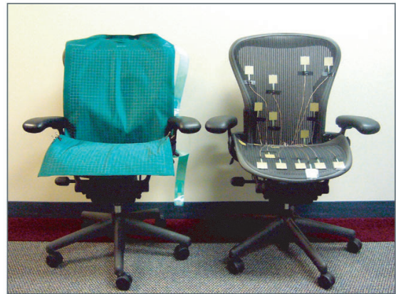
Figure 1: On the left is the commercially-available Tekscan ConforMat system (2048 sensors) installed on a Herman Miller Aeron Chair. On the right is our deployed system (19 sensors) installed on the same model of chair.
