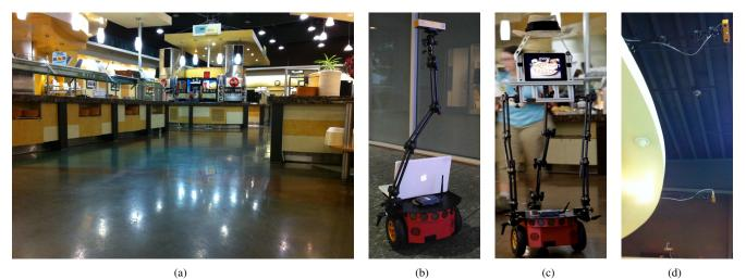
Fig. 3. (a) The robot workspace consists of a  $20m^2$  area surrounded by a buffet (left), a pizza station (right), and a soda fountain (background). Distance between start and goal was 6m. (b) Old form factor (c) New form factor (d) 3 overhead stereo cameras comprising the tracker.
